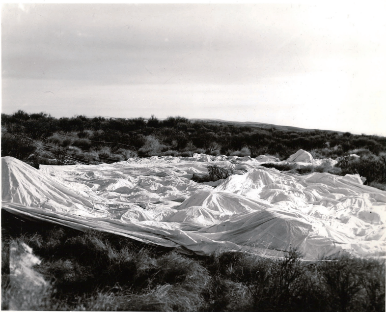
#15 - Prosser Balloqn - Section of bag, as found. (Note ice which has formed.)
